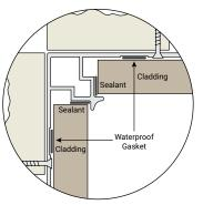
(12 x 10mm inner foam gaskets optional, alternative sealant option)
