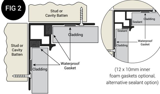
**Aluminium Internal Corner Stop (install prior to cladding)**
