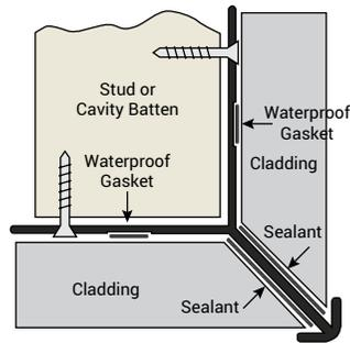
**Aluminium External Corner Stop (install prior to cladding)**
