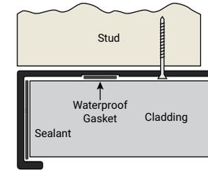
**Aluminium End Stop L (install prior to cladding)**
