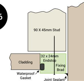
**Timber End Stop (install prior to cladding)**
