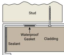
**Aluminium End Stop L (install prior to cladding)**
