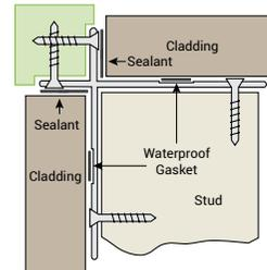
**External Cross with Timber Corner (install prior to cladding)**
