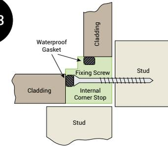
**Timber Internal Corner Stop (install prior to cladding)**
