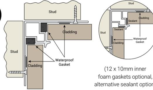
(12 x 10mm inner foam gaskets optional, alternative sealant option)
